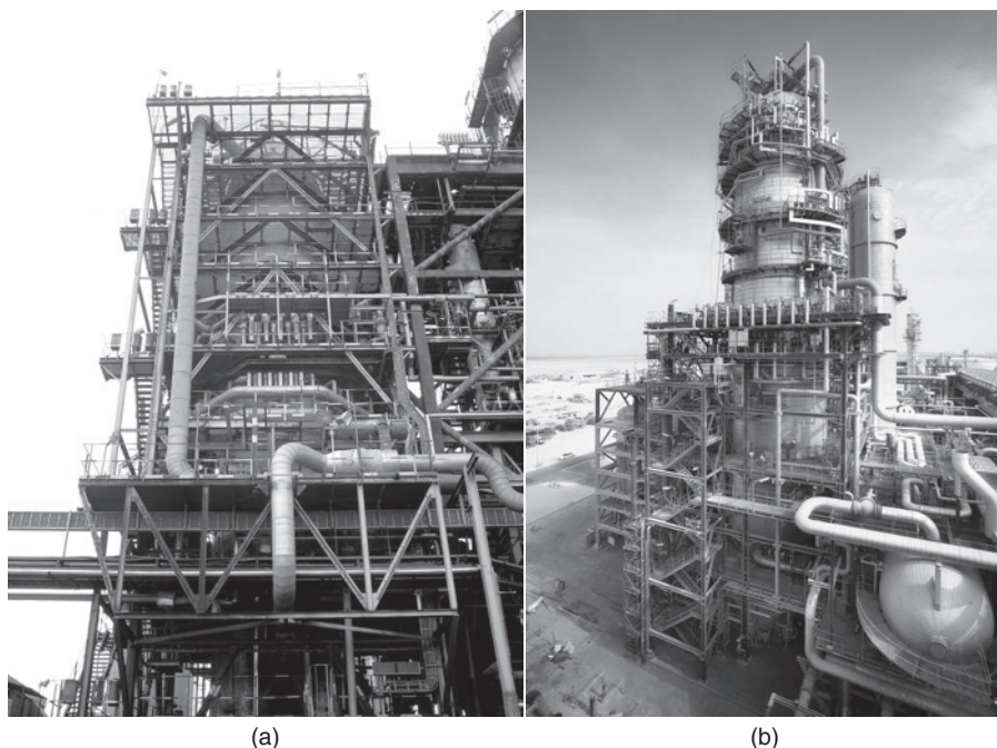
Figure 1.16. (a) Sasol's 5-m ID F-T reactor for coal-to-liquid synthesis. (b) Sasol's Oryx gas-to-liquid plant in Qatar, which consists of two low-temperature Fischer–Tropsch SPD (slurry-phase distillate) reactors with a capacity of 17,000 bbl/d each, producing a primary product of low-sulfur diesel oil using the feedstock of reformed natural gas. It shows one reactor of 10-m ID in front, with another of the same size behind it. Photo: courtesy of Sasol Limited.
